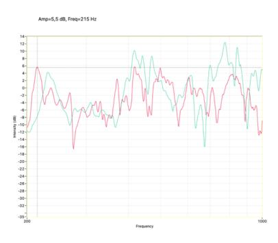
Figure 4: The Helmholtz air resonance on a Viola a chiavi di Siena is 215Hz.
