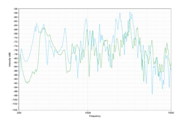
Figure 1: Green describes the instrument right after finishing and the blue graph was measured after two years of playing.
