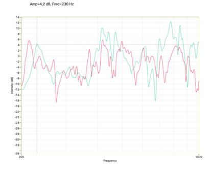
Figure 5: The Helmholtz air resonance A0 on a 40.5cm long Viola is 230Hz.
